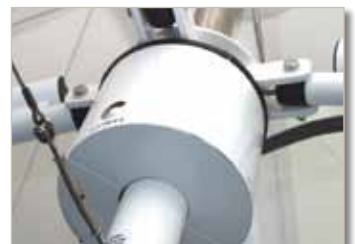
Wiring loom access cover
